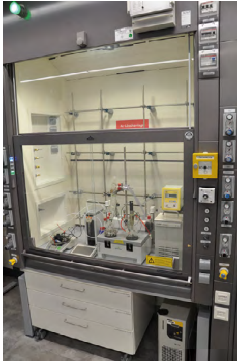
Fig. 1: Height-adjustable fume hood with knee space. The cabinets are on wheels and can be removed as needed to make room for a seated person (in a wheelchair). The important controls can be reached from a seated position. The ventilation system is not only equipped with an acoustic alarm signal, but also with two visual alerts (at eye level and above the sash). In addition, a person working at this unit is given a mobile safety device for single-user workplaces with an alarm button that is accessible at all times.
