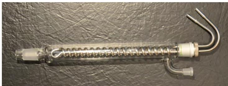
Fig. 16: Condenser with metal condensing coil inserted
