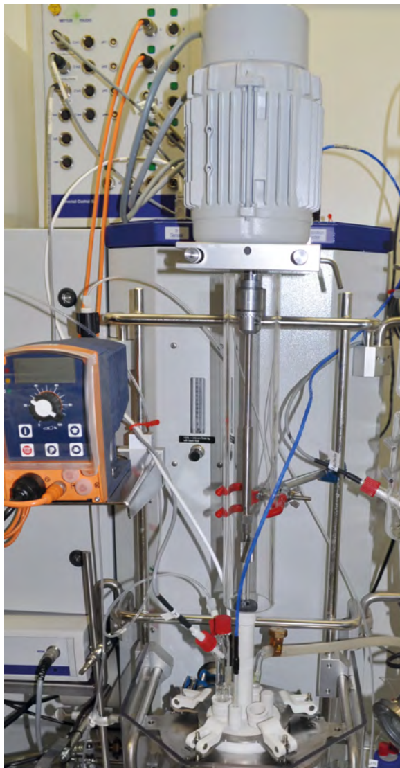
Fig. 23: Laboratory stirrer with protective plastic sleeve
