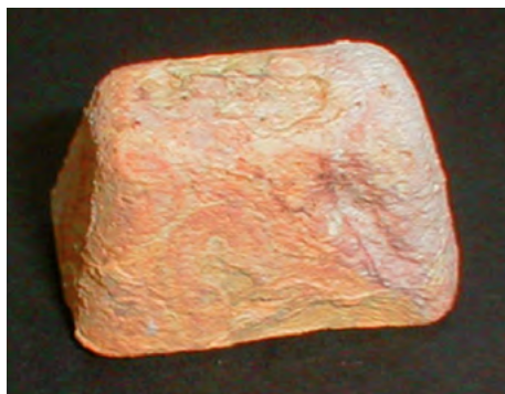
Fig. 11: A highly oxidized piece of potassium (21)
