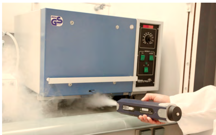
Fig. 12: Examination of the flow conditions of a jacked-up furnace in a fume hood using a handheld fog generator
