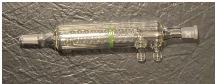
Fig. 13: Condenser with glass screw threads for cooling water connection
