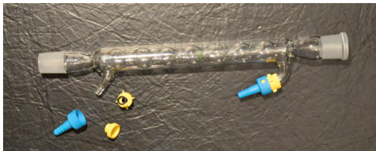
Fig. 14: Condenser with glass olives for cooling water connection with adapters for retrofitting plastic quick-action couplings
