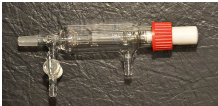
Fig. 20: Overpressure valve for glass apparatus
