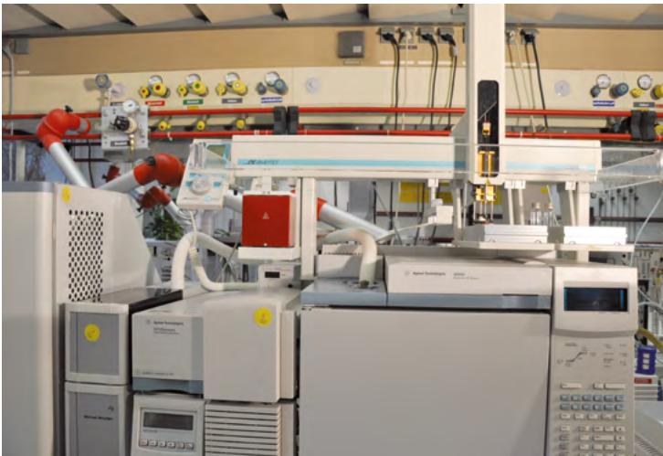
Fig. 29: Example of a local extraction device on a gas chromatograph
