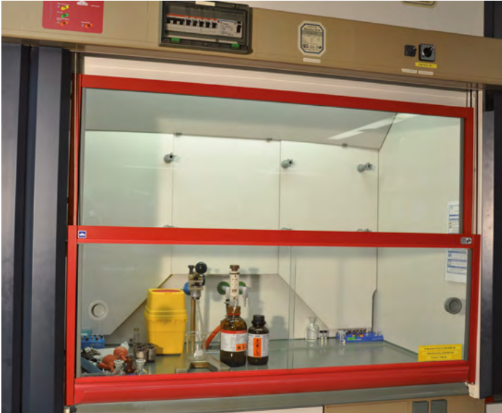
Fig. 30: Fume hood with divided sash
