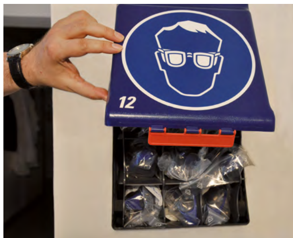
Fig. 3: Storage box for safety glasses for visitors at the entrance to a laboratory area; glasses are cleaned after use and kept in plastic bags
