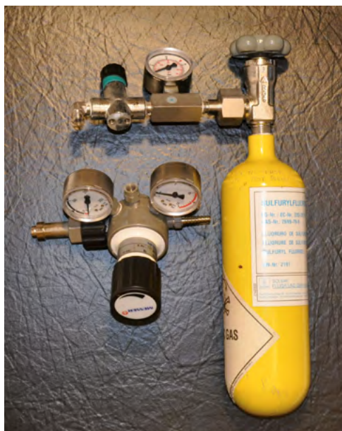
Fig. 21: Pressure reducer and needle valve (on the cylinder)
