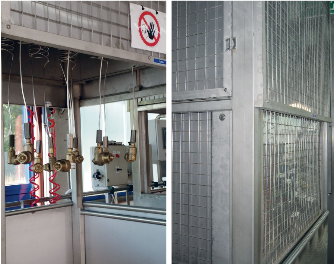
Figure 1: Shielding of a Filling Station, open (left) and closed (right)
