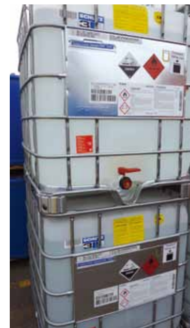
Chemicals should be stored in original containers
