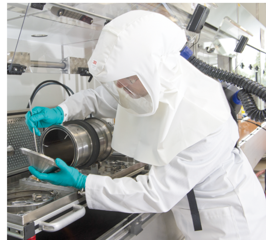
Personal protection for working with special nanomaterials.
