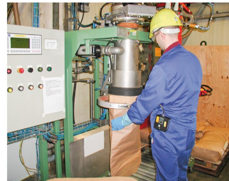
Personal air monitoring to assess the effectiveness of the ventilation system
