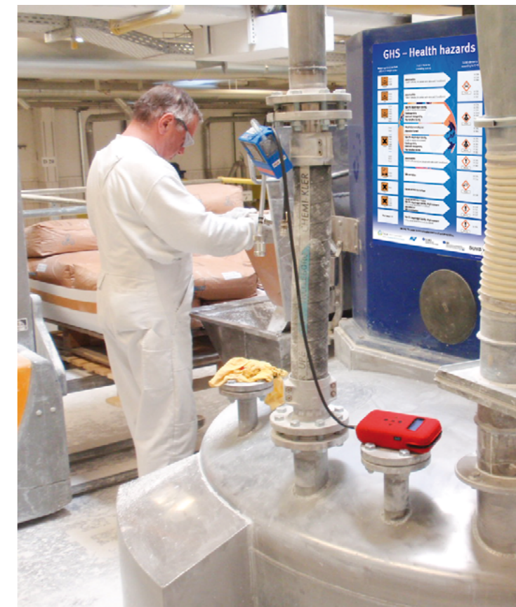
Stationary dust monitoring during filling process
