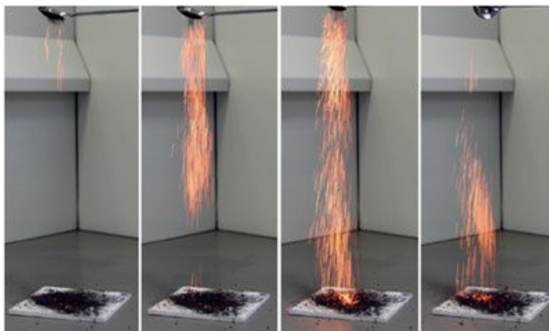
Figure 26: Positive test for pyrogenic properties with n-iron (50–70 nm)
