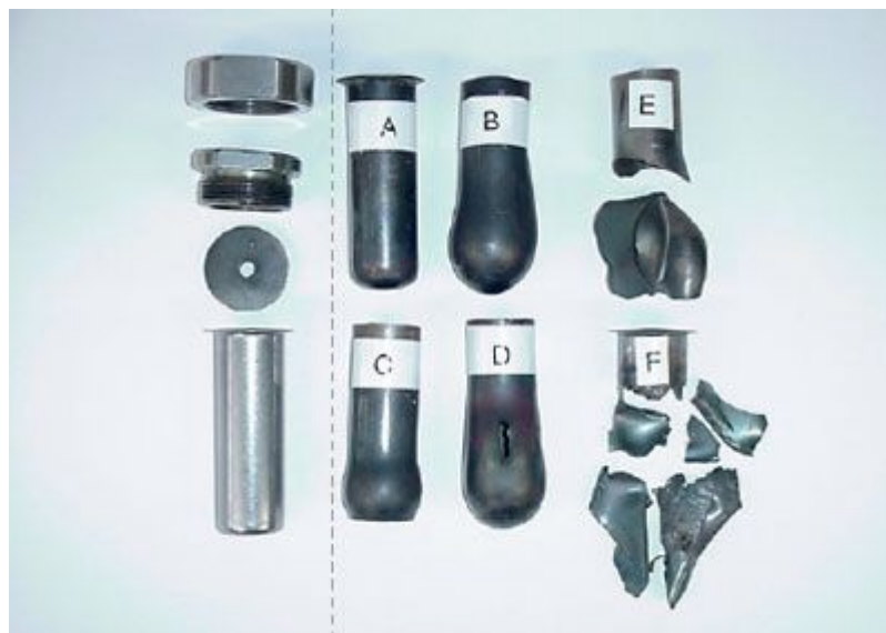
Figure 5: Left: intact steel tube before the test. Right: deformed or shattered tubes after the test
