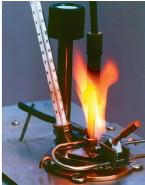
Figure 20: Flash point test in a closed cup (a large flame only occurs way above the flash point)
