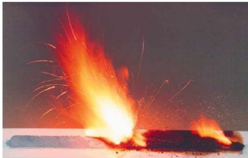
Figure 25: Measurement of the burning time of a powder train
