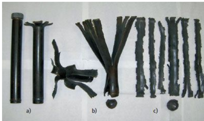
Figure 14: Fragmentation after a 2" steel tube test a) No propagation b) Partial propagation c) Complete propagation
