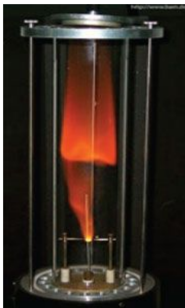
Figure 16: Determination of the explosion limits of ammonia (tube method) according to DIN EN 1839
