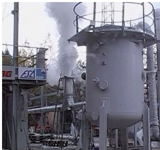
Figure 8: Explosion isolation using explosion diverter
