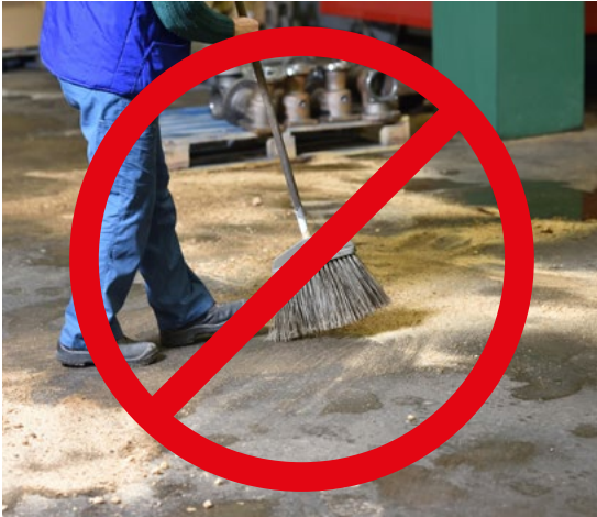
Figure 5: Unsuitable process (left) and suitable process (right) for the removal of combustible dust
