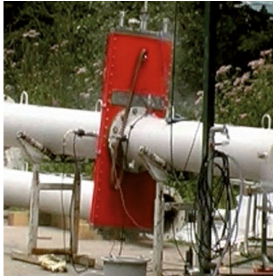
Figure 7: Explosion isolation using rapid-action valve
